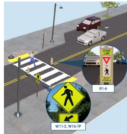
Crosswalk Visibility Enhancements
